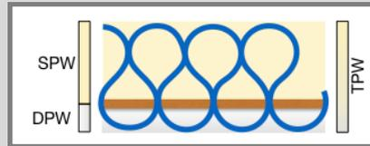
The surface pile weight is the technical relevant value according to EN 1307 and has to be mentioned in technical specification. As shown in the figure below alternatively to the total pile weight the surface pile weight can be used to calculate LCA results (IC<sub>x</sub>).
